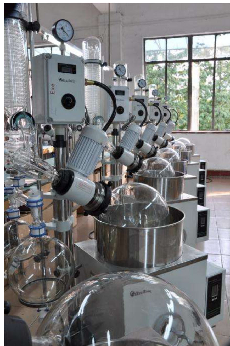
Pilot Scale Rotary Evaporator
